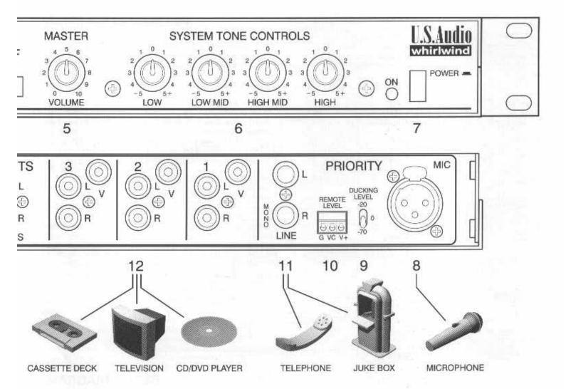
ng the tonality of a sound system HIGH are bass and treble shelving set at 250 Hz and 1.6 kHz.
